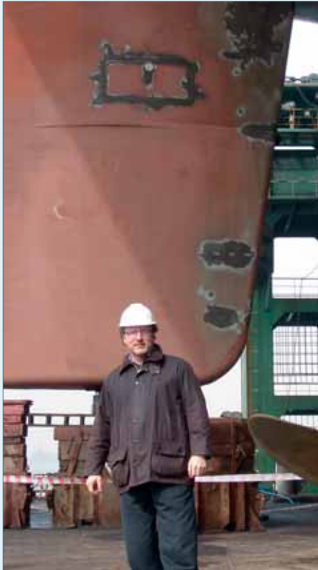
Mr. Kuhlmann inspecting a TLKSR® Twisted Rudder at a Chinese dry dock following 5 years of operation
