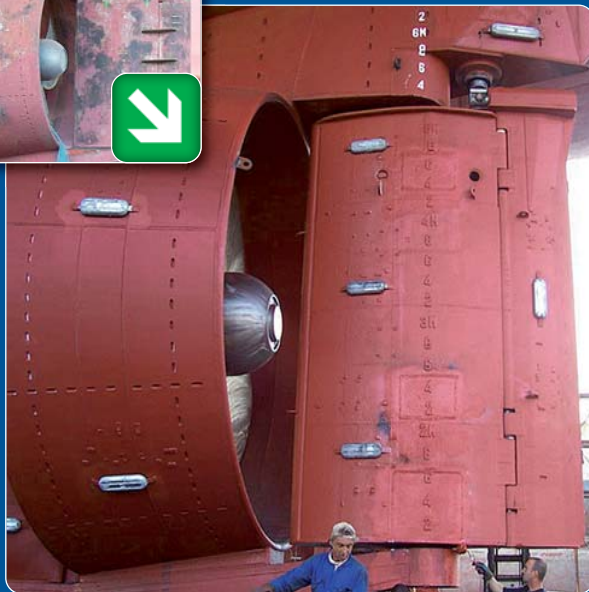
e.g. new linkage system retrofitted on 18 years old Flap Rudders of stern-trawlers.
